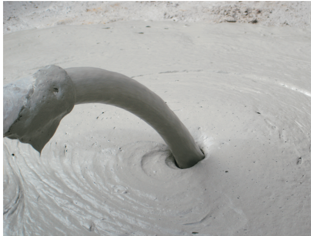
Flowable properties of cellular concrete
